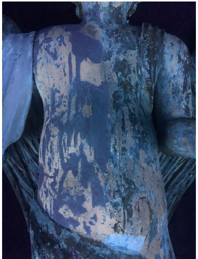
Figure 3: The torso in UV light. The fillings fluoresce dull greyish purple, the paint orange, and the chalk ground white.
